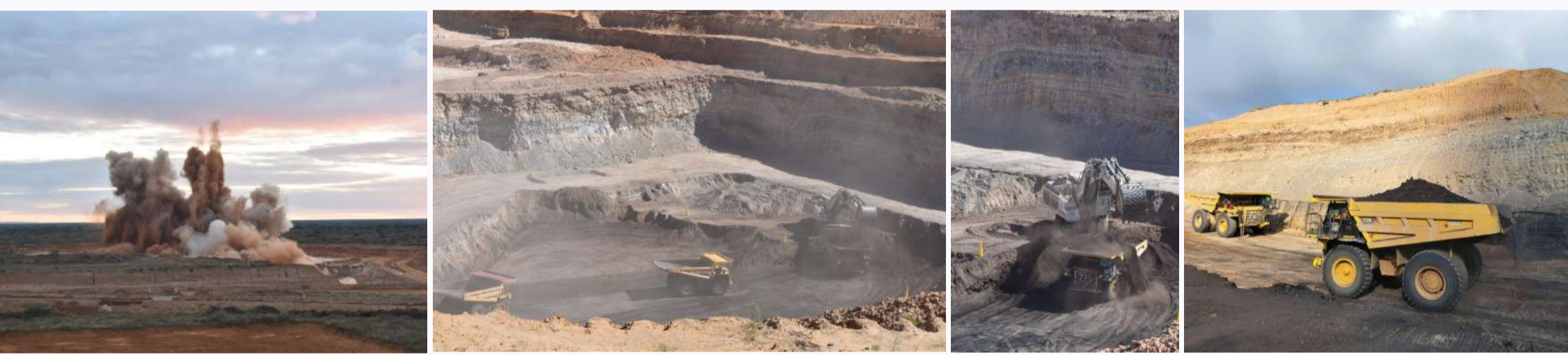
Mining students from BIUST visited MCM Another milestone for MCM at the opencast mine as the first coal has been exposed after safely conducting 20 blasts. The Box-cut is 40 meters deep now and No. 2 Seam coal has been intercepted. This weathered coal will be used to dress the ROM pad as well as the slow conveyor discharge area, in preparation to receive the main coal. Mining of overburden will continue as more waste have to be moved to expose the main coal.
